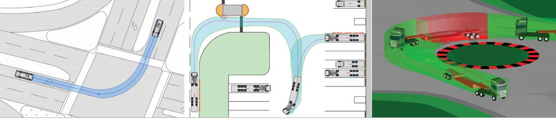
Great for checking vehicle maneuvers in simple environments, such as passenger vehicle turns in parking lots and intersections
